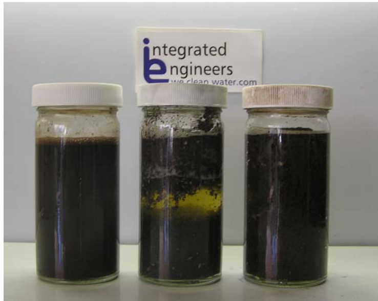
Untreated (left), Treated with Floccin 909 (center) with slight organic coloring remaining.
